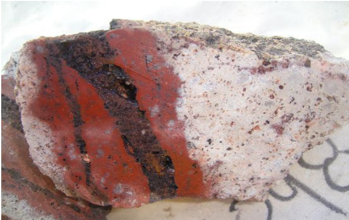
Image 2. Sample #3004098 Bleached sericite altered rhyolite porphyry. cut by gossanous vein with ferruginous selvage.
