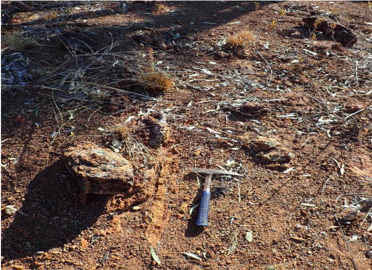
Image 4. Sample #3004086 Sulphate vein cutting sericite altered rhyolite porphyry.
