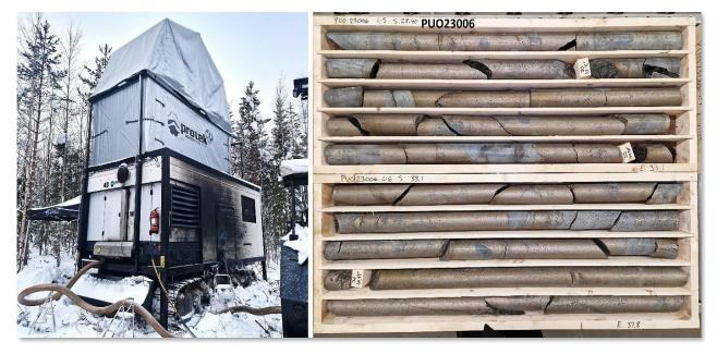
*Figure 2:* Image of the drilling rig on-site at Puolalaki and massive sulphide mineralisation in drillhole PUO23006, (28.4-37.8m).
