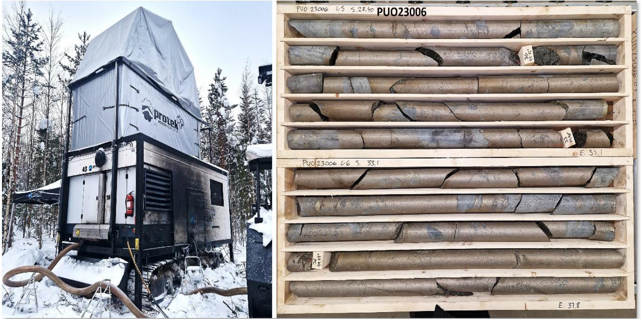
Figure 3: Photograph of the drilling rig on-site at Puolalaki and massive sulphide mineralisation in drillhole PUO23006, (28.4-37.8m).
