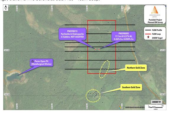
Figure 4: Planed FLEM profile and Loop with the tenement area
