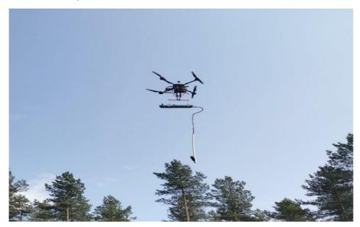
Figure 3: Image of Drone MAG system
