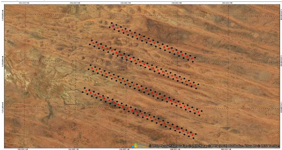
Figure 4: MLTEM Surveying completed at the Mt McPherson project
