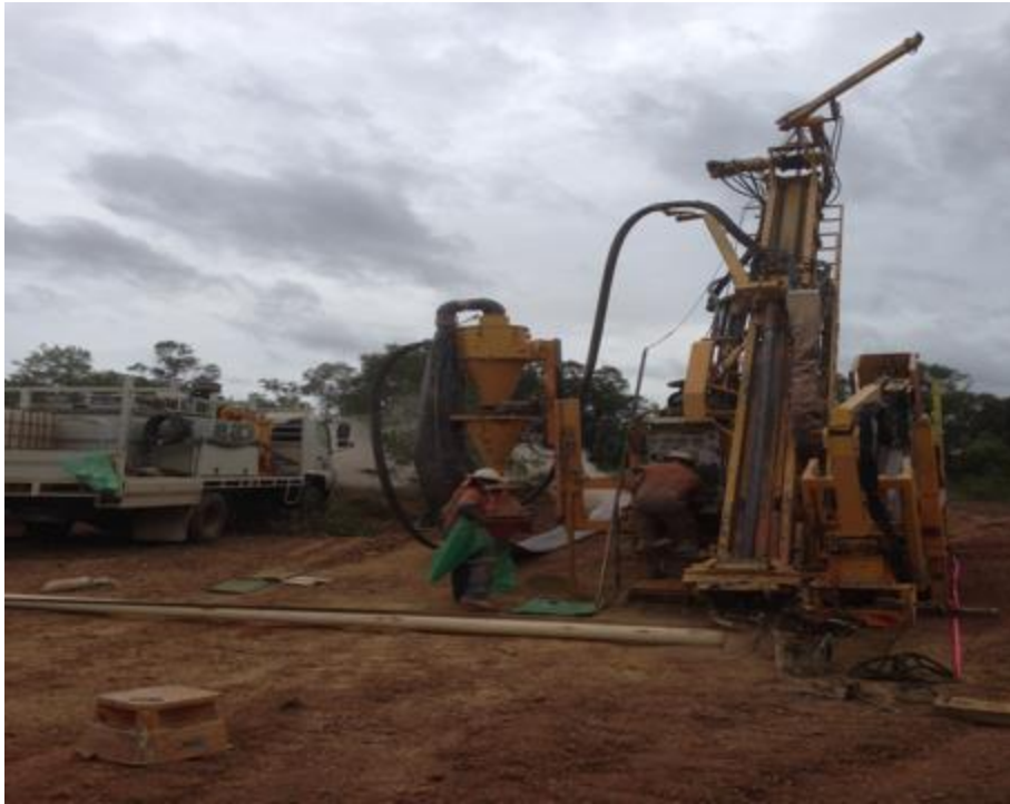
IMAGE 2. Reverse circulation rig commencing RC drill hole at Pyramid
