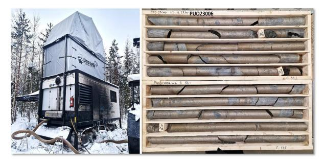
**Figure 7**: Drilling rig on-site at Puolalaki and massive sulphide mineralisation in drillhole PUO23006, (28.4-37.8m).
